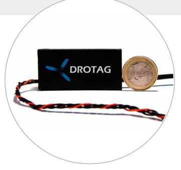
**DroTag** is a small board that simply sits between your **CHDK capable** camera and your **Pixhawk**, allowing you to plan the camera trigger events and have the **pictures taken automatically geo-tagged on the fly**.
